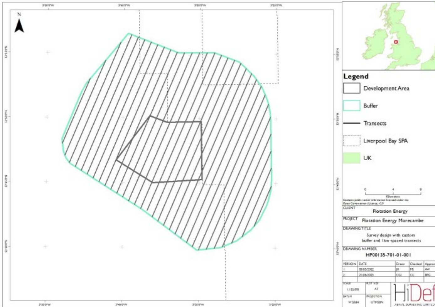
Plate 3.1 Morecambe survey design with 4-10km hybrid buffer with 1km-spaced transects flown between March 2021 and February 2023
